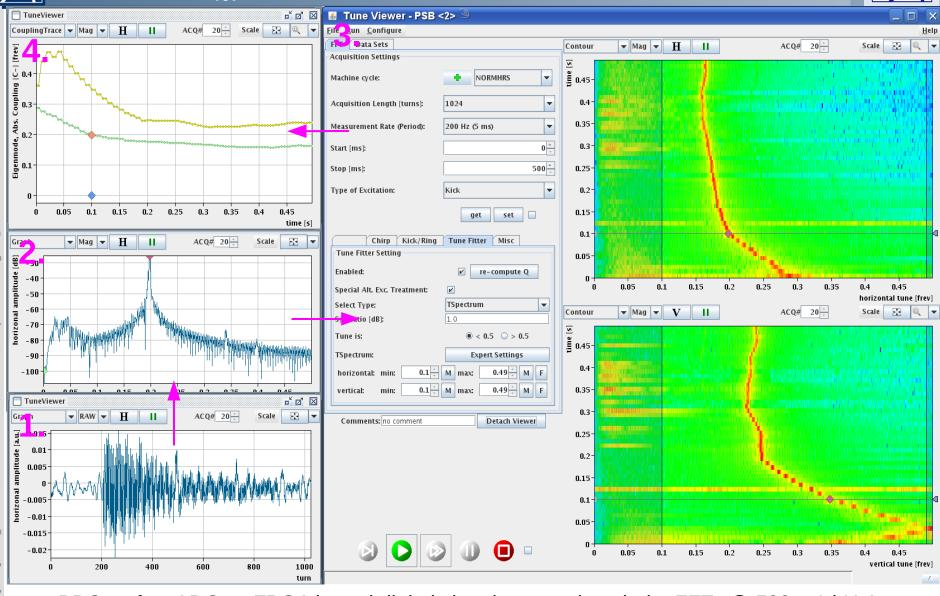
BBQ  $\rightarrow$  fast ADC  $\rightarrow$  FPGA based digital signal processing chain, FFTs @ 500 – 1 kHz! – provides real-time Q diagnostics for operation
